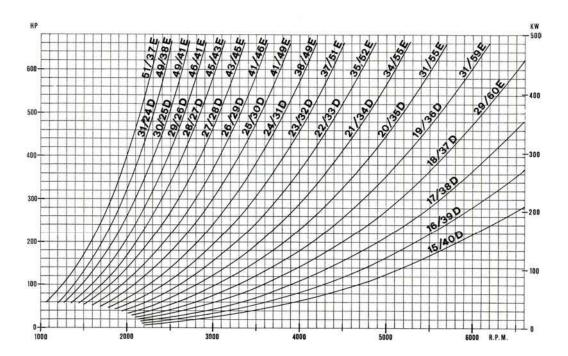
The above curves show the power absorption characteristics for the range of gear wheels ratio available. The engine maximum flywheel power/r.p.m. output should lie within the area between 51/37 and 15/40 ratio.
