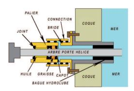
Hydraulic Seal Patent: oil circulation, double dry stage, self-aligning bearing.
