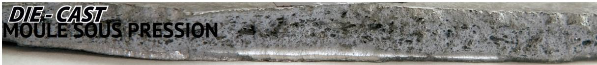
PROCÉDÉ DE LA CONCURRENCE : TROUS, BULLES D'AIR - FAIBLE ET FLEXIBLE - TRANSFERT DE PUISSANCE INEFFICACE - RAREMENT REPARABLE
